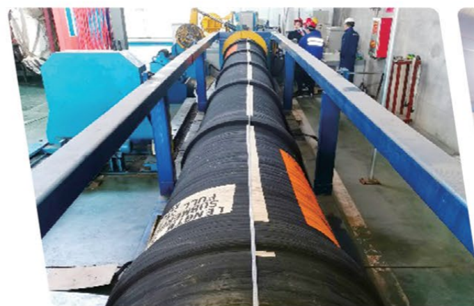
24 寸水下油管拉伸试验 Tensile test of 24 inch submarine hose
