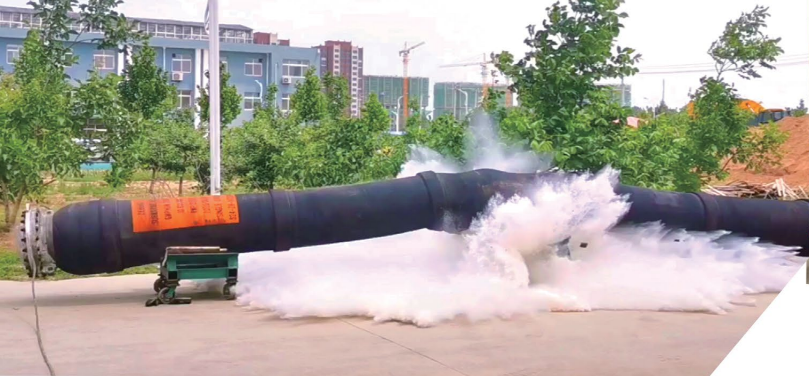
泽邦生产的水下油管爆破试验 Bursting pressure test for submarine oil hose by Zebung
