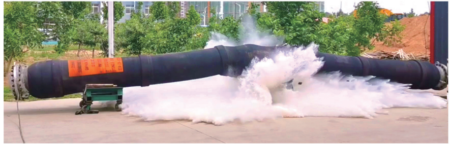
水下油管爆破试验 Bursting pressure test for submarine oil hose
